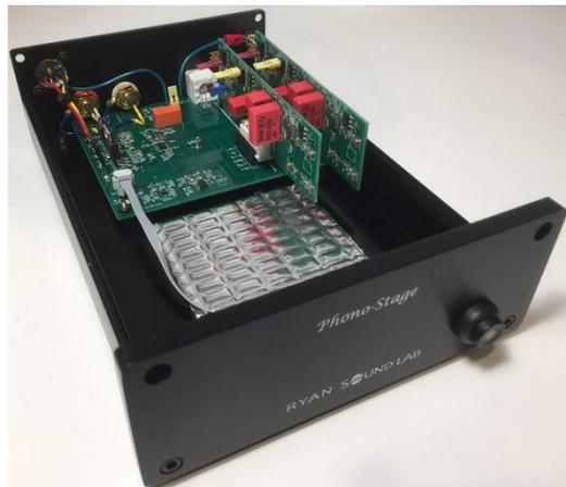
new ones making sure the connector pins all line up. An Allen wrench is provided for removing the two front top screws while a standard Phillips screwdriver is needed for the rear panel top two screws to allow removal of the case top section to gain access to the plug-in boards.
